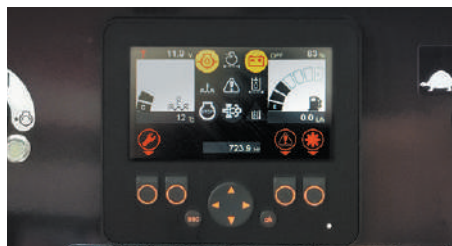
Multi-function Display shows RPMs, fuel, service alerts, and error logs.
