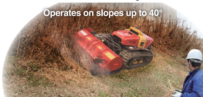
Flail Head with Floating Deck
